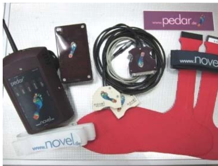
Figure 1. Pedar in-shoe pressure measurement system
